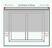
When face fitting the brackets, (usually on Exact Size), ensure the B distance in the diagram on the left is the same on both sides of the window, so that you can have an uneven overlapping.
