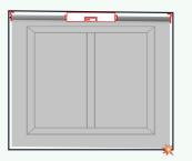
When top fixing the brackets, to avoid installing your blinds tilted, ensure the lintel or ceiling are levelled using a spirit level. If not, put a paper between one of the brackets and the ceiling or lintel to compensate the inclination on both sides.
